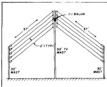
fig. 1. The 80-meter wideband dipole at W7IS.
