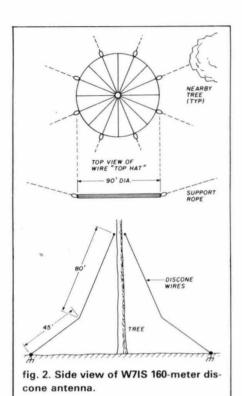
into position at the 80-foot level! He used nylon ropes to steady the assembly. The ropes ran to seven nearby trees. Pulleys and weights on each of the ropes allowed the top disc to flex in the wind.
